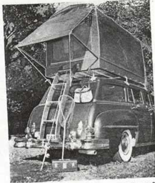
Ladder leading to entrance has curved stiles to fit over car trunk. Ladder is hinged to car bumper
